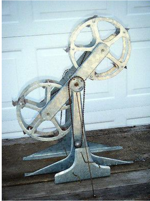
Figure 12: Chain Driven Double Ferris Wheel [12]
